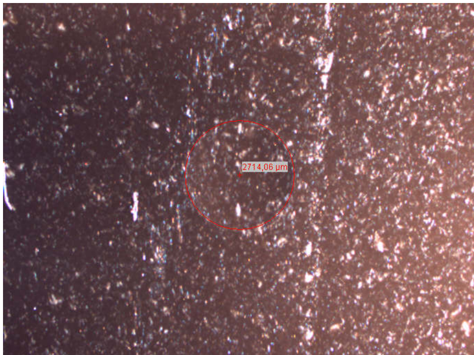
Figure 2: microscope image of the Brinell hardness-indentation on the bottom
